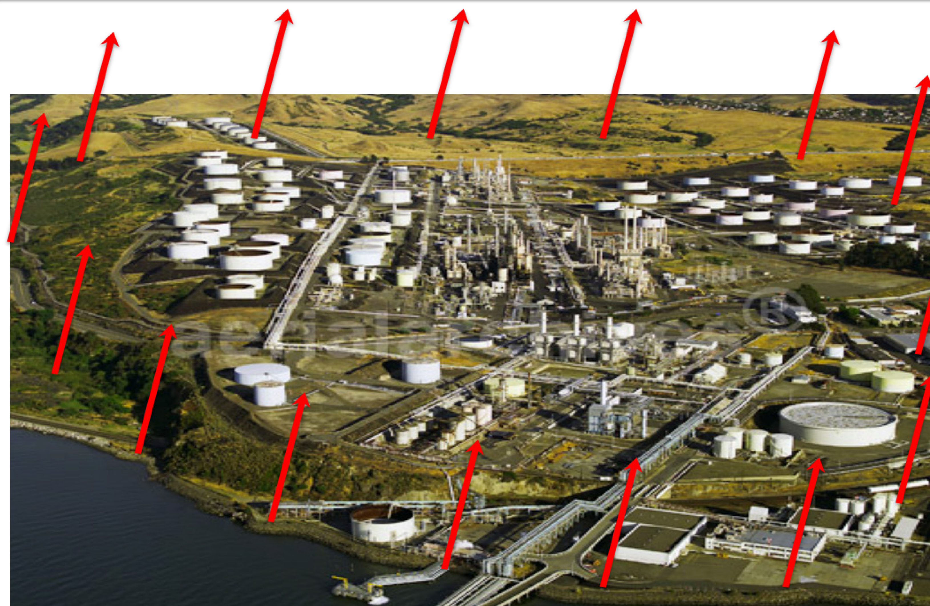
Figure 3. A GHAPS Wide Area Monitoring System. Autonomous GHAPS sensors can form perimeter monitoring systems. Red arrows illustrate placement of GHAPS instruments monitoring emission from refinery.
